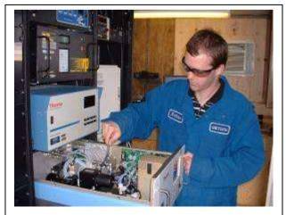
An Ortech Environmental field consultant services a sulphur dioxide air quality monitor at an SLEA's monitoring station, as part of an ongoing instrumentation maintenance program. Reliable service and accurate data are hallmarks of the associ-ation's monitoring network.
