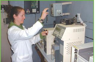
ORTECH Environmental laboratory technician Lisa Nauta checks the accuracy of the water quality monitor at the Sarnia-Lambton Environmental Association's St. Clair River station, near Courtright.
